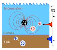
For material samples, where surface functionalities are of the main interest, the signal of **the bulk must be separated from the signal of atoms localized on the material surface.**
